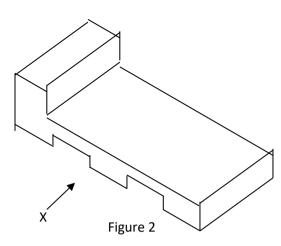
24) Which of the following represents the front elevation in the direction of the arrow X?
