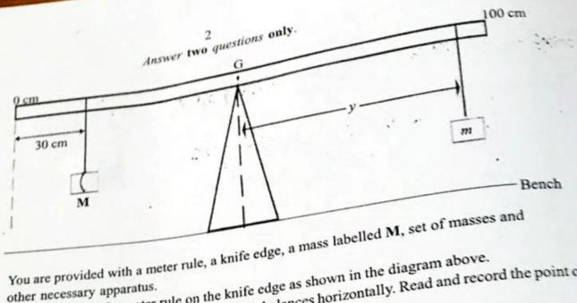
Suspend the meter rule on the knife edge as shown in the diagram above. Adjust the position of the rule until it balances horizontally. Read and record the point of other necessary apparatus.
