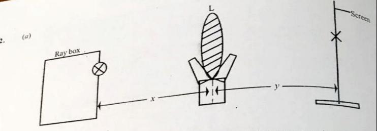
You are provided with a ray box, a converging lens L, a lens holder, a meter rule, a screen and Place the lens L in its holder, and move it towards or away from the screen until other necessary apparatuses.
